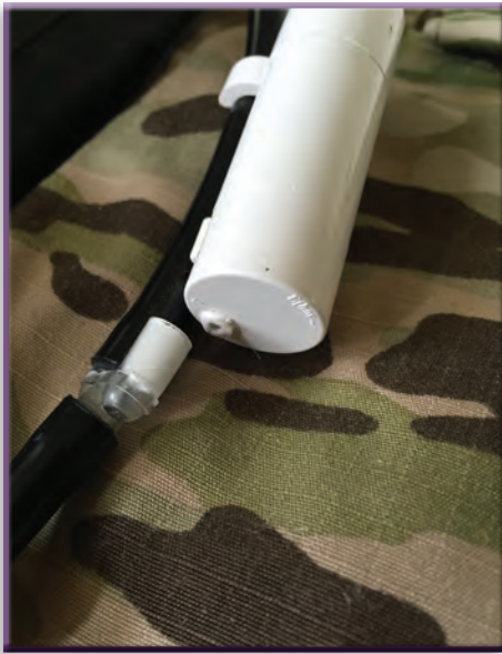
Figure 1 Breakage of gauge from repetitive stress.
